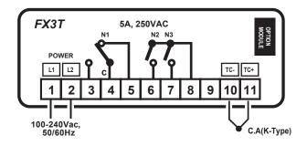
OUT1: HEAT/COOL#1 ON/OFF output, Alarm output
