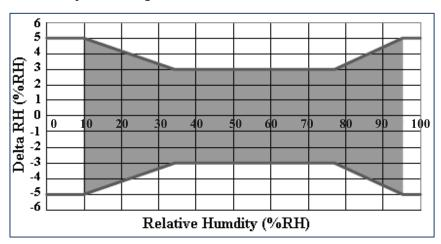
HTX3515 modules are specified for maximum accuracy measurements within 10 to 95 %RH.
